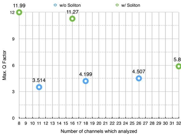
Fig. 6. Comparison performance with and without soliton
