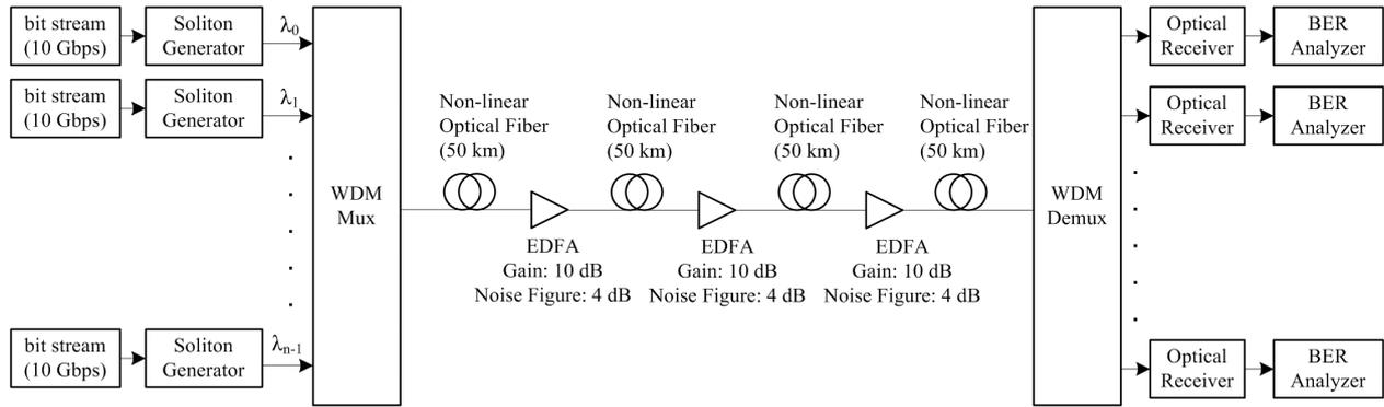
Fig. 1. Soliton Transmission DWDM System Over Non-linear Optical Fiber [8]
