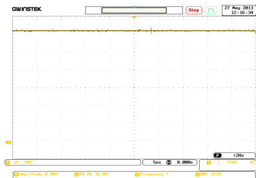
(b) Boost-up chopper output voltage
