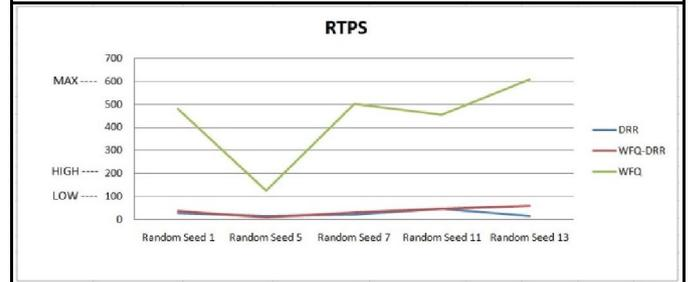
Curve B. Delay comparison DRR, WFQ-DRR, and WFQ for rtPS
