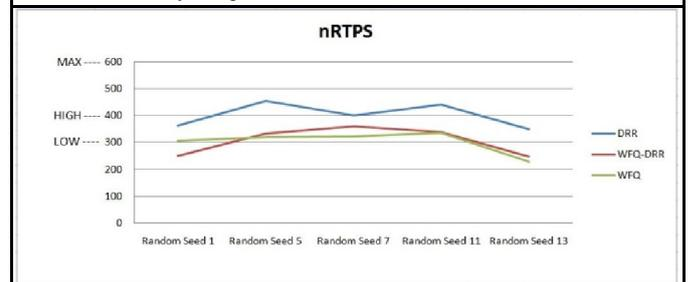
Curve D. Delay comparison DRR, WFQ-DRR, and WFQ for nRTPS
