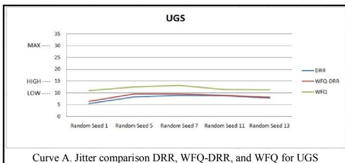
Curve A. Jitter comparison DRR, WFQ-DRR, and WFQ for UGS
