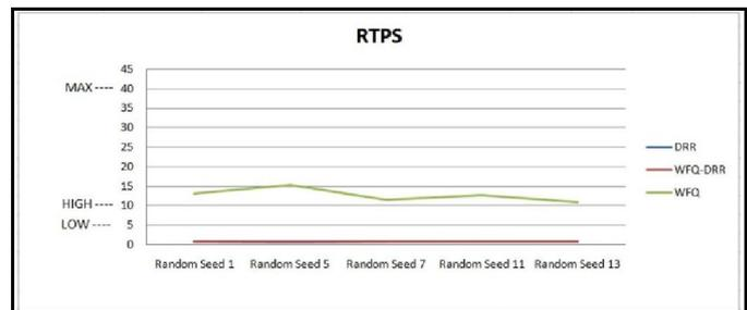
Curve B. Jitter comparison DRR, WFQ-DRR, and WFQ for RTPS
