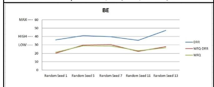
Curve E. Jitter comparison DRR, WFQ-DRR, and WFQ for BE
