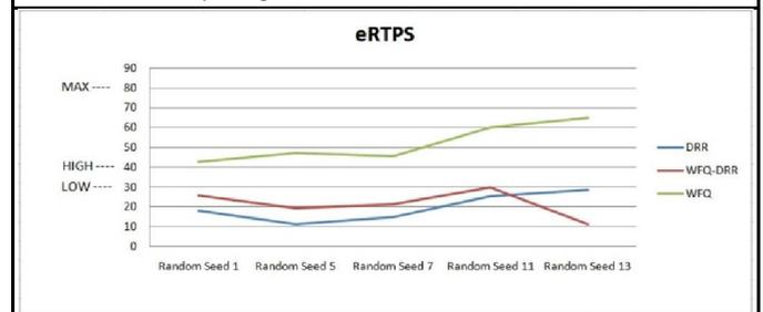
Curve C. Delay comparison DRR, WFQ-DRR, and WFQ for eRTPS
