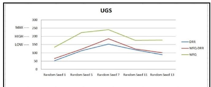
Curve A. Delay comparison DRR, WFQ-DRR, and WFQ for UGS
