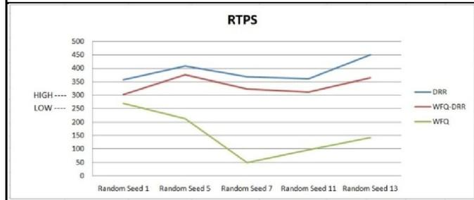
Curve B. Throughput comparison DRR, WFQ-DRR, and WFQ for rtPS
