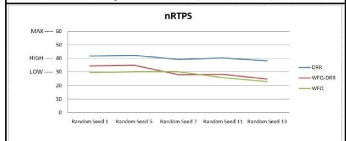
Curve D. Jitter comparison DRR, WFQ-DRR, and WFQ for nRTPS
