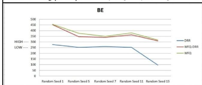
Curve E. Throughput comparison DRR, WFQ-DRR, and WFQ for BE
